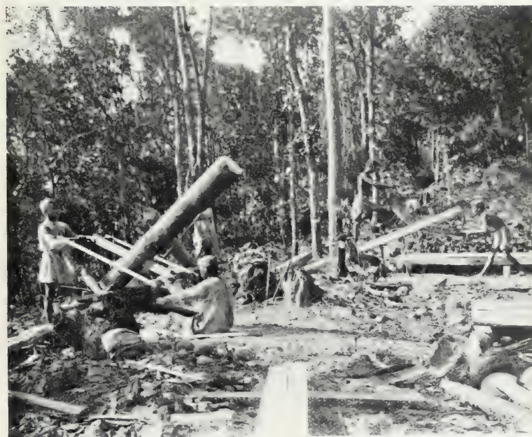
FIG. 149. NATIVES SAWING WITH FRAME AND DELHI SAW : INDIA. [Photo : R. S. Truof.]
